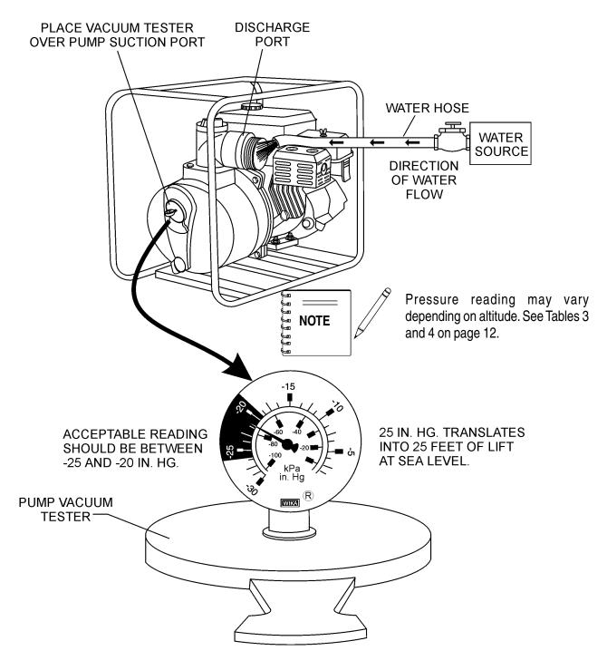
Figure 17. Pump Vacuum Tester
